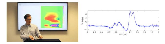
**Figure 1**. The image on the left demonstrates one visualization of spatially continuous strain data acquired by Sensuron's fiber optic sensing platforms. The x-axis represents length along the fiber, the y-axis represents time and the colors represent strain measurements. This is in contrast to the image on the right which is the strain output from a single strain gauge where one point of data is collected over time.
